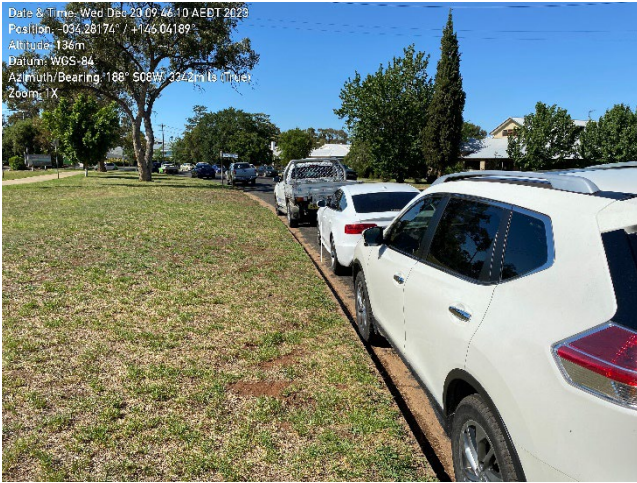
Sedimentation in the gutter down-gradient of the site access on Animoo Avenue.
